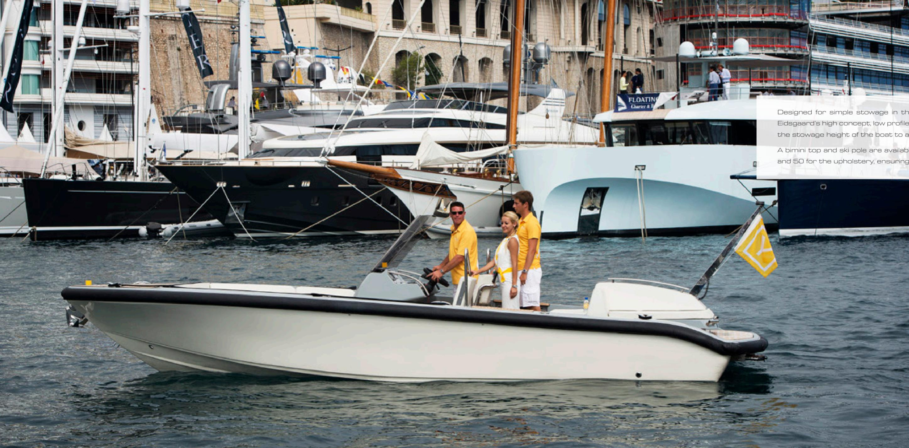
Designed for simple stowage in the side or stern garages of 45 to 50 meter motor yachts, Eidsgaard's high concept, low profile design features a unique, offset folding console which reduces the stowage height of the boat to a mere 1.51m.
