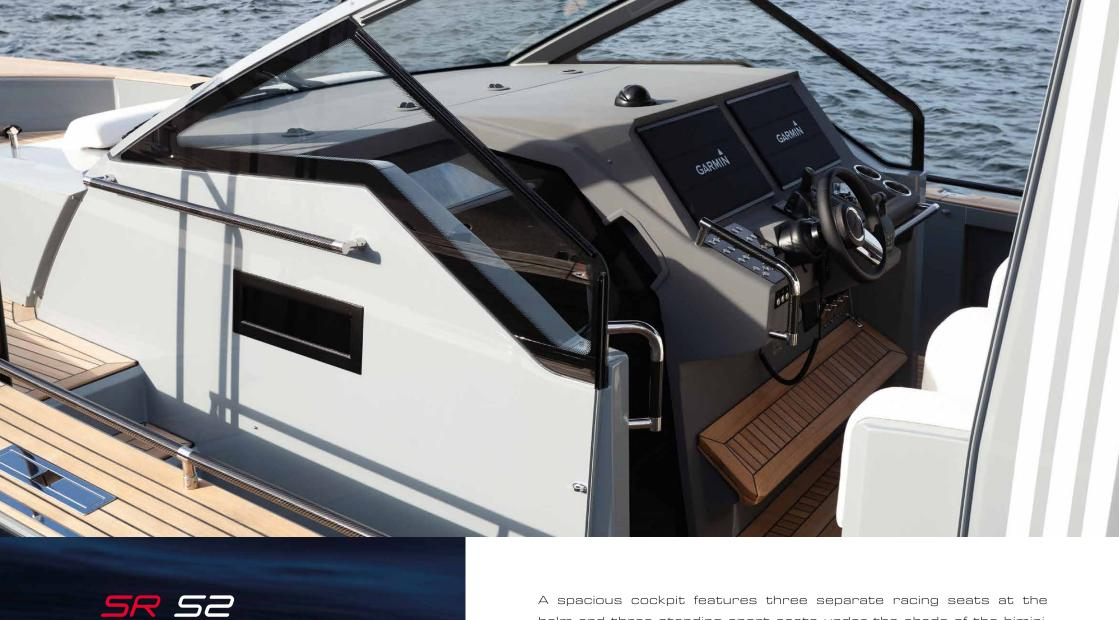
A spacious cockpit features three separate racing seats at the helm and three standing sport seats under the shade of the bimini. The teak deck provides open walkaround access from the raised foredeck to the additional seating, sun lounger and hydraulic bathing ladder aft - perfect for race spectating, swimming or picnicking at anchorage. A head with shower is located below decks, along with a double berth. Truly, a superyacht among tenders.
